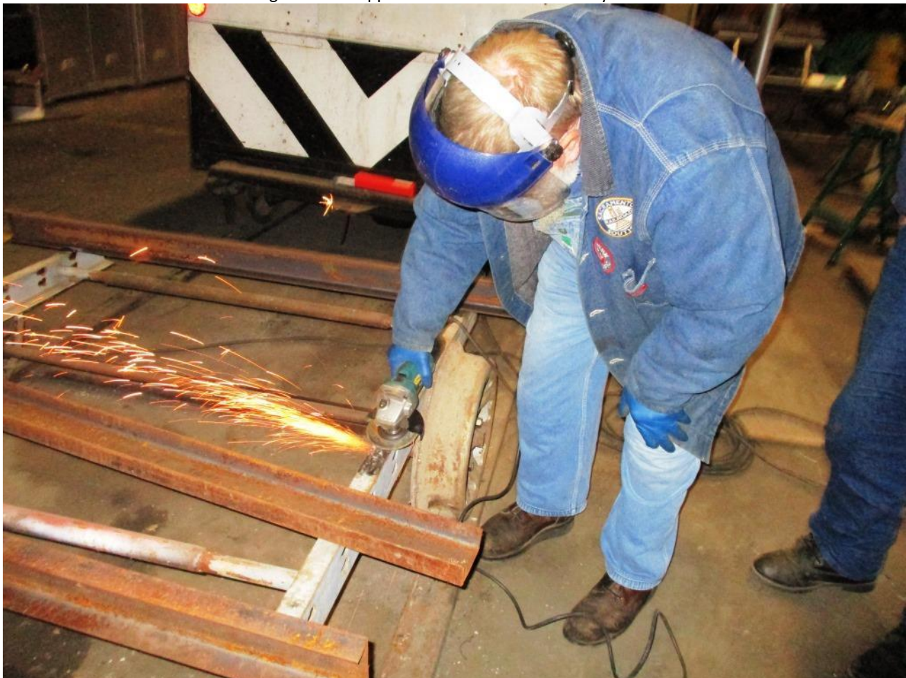
Pat grinding down the weld on the new hydraulic-tool car
