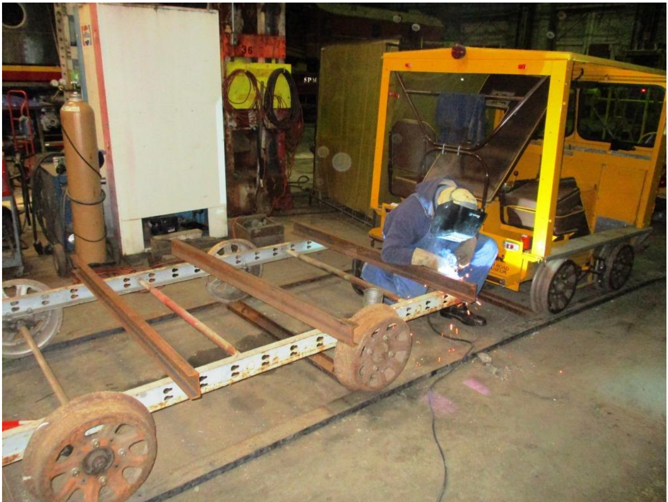
Cliff welding the deck supports for our new dedicated hydraulic-tool car
