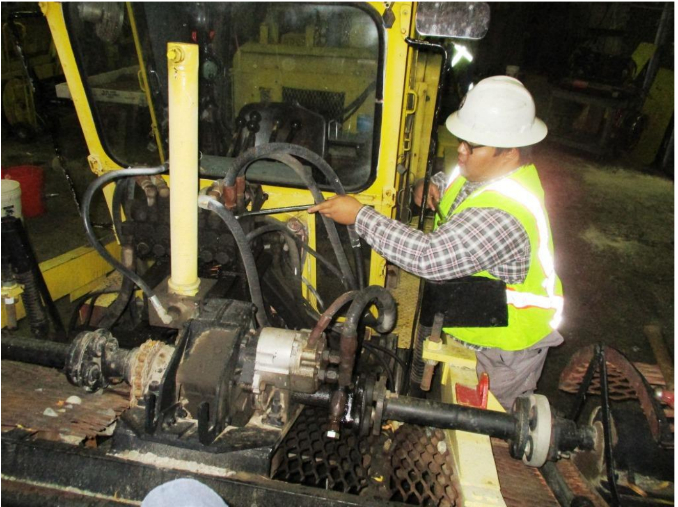
Anthony caps the hydraulic receptacle on the scarifier
