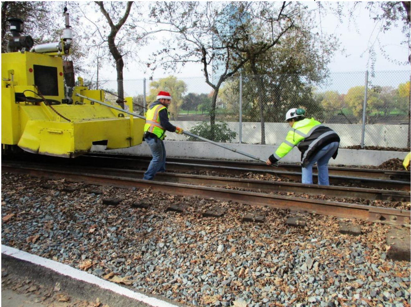
Following the 125's hydraulic cylinder calamity, Joe and Pam use the long draw-bar to connect the regulator to the 125 for towing
