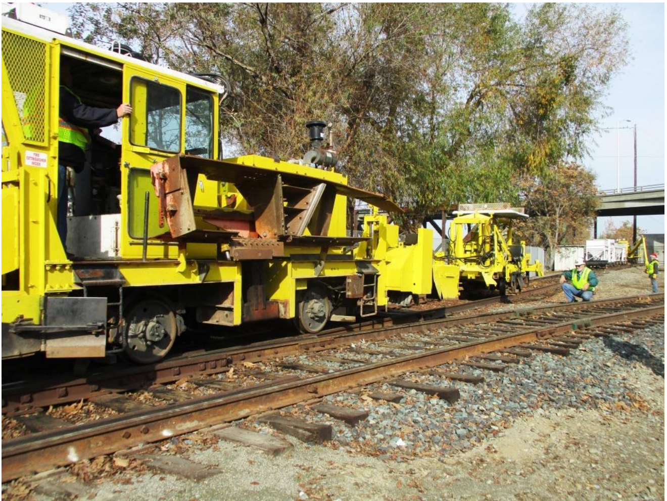
Chris C. in the regulator shoves the 125 while Alan watches closely to make sure its descended turntable doesn't hang-up on anything else
